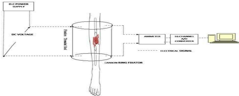
Figure 2: Experimental set-up for fracture healing model analysis
